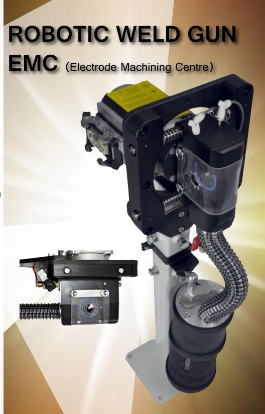
The specific design combines synergistic motor power (nominal 1HP), gearing and output rotational speed (680rpm) at the cutter location, together with a highly defined, reliable single (HSS with newly developed coating technology), or four blade (New Generation Carbide), cutter technology. All Cutters conform to RWMA specifications.
